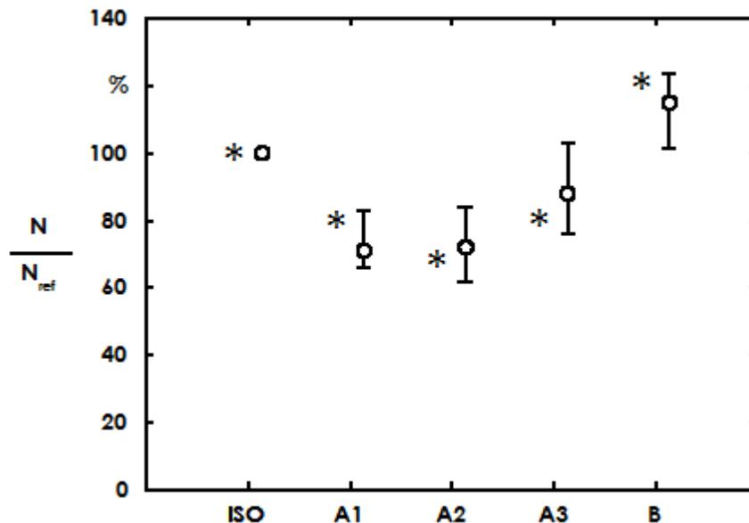
Figure 1-Loudness of pass-by sounds from a passenger car at 50 km/h in 7.5 m distance for a “normal” tire on different road surfaces. ISO represents the ISO10844 road surface; A1, A2, A3 stand for three different sound absorbing road surfaces, and B for a conventional, non-absorbing road surface. Data from psychoacoustic experiments (circles) in comparison to physically measured values of percentile loudness  $N_5$  (stars)
