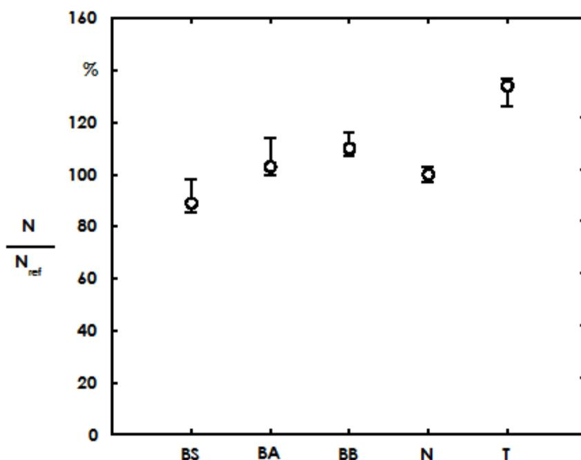
Figure 2-Loudness of pass-by sounds from a passenger car at 50 km/h in 7.5 m distance for different tires on the sound absorbing road surface A 2. BS broad tire without tread (slick); BA and BB broad tires with different tread; N “normal” tire; T tire of a truck.
