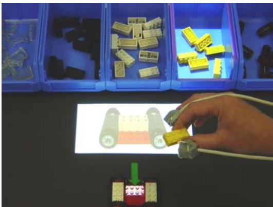
Figure 2 A video overlay method for presenting task instruction and registration of a grasping movement using the Polhemus marker system.
