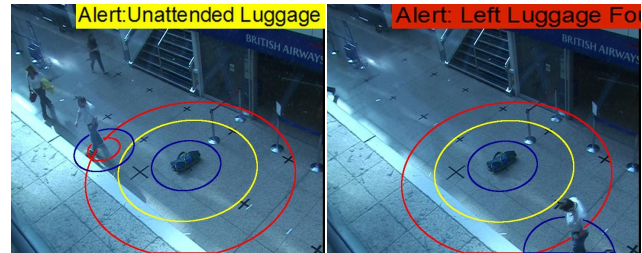
Figure 11: A sample from S08. First the person leaves the 3m radius. After 25s an alert will be set
