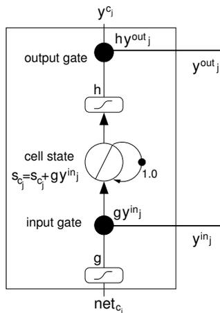
Fig. 2. A memory cell of a LSTM-RNN.
