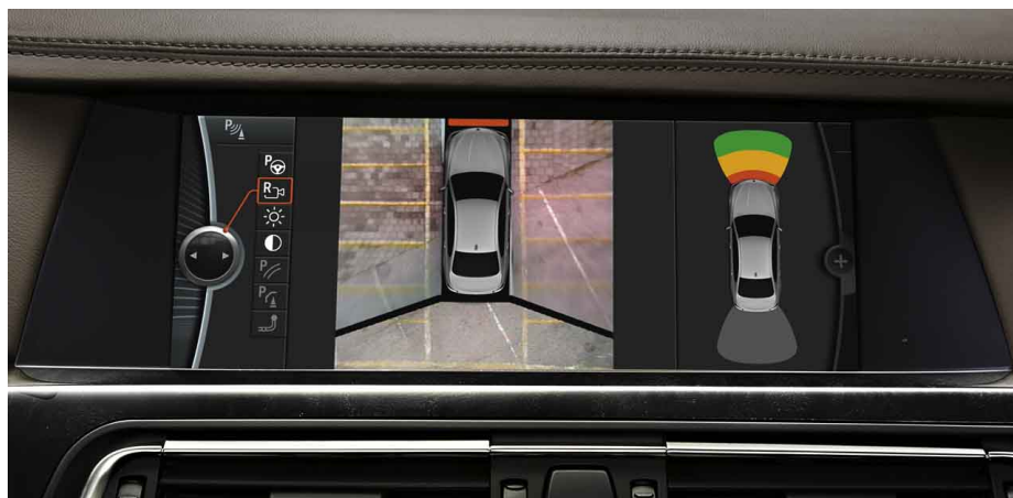
(f) User interface: the images of the top-view and backward-looking cameras are undistorted and displayed together.
