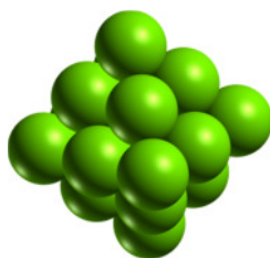
Figure 5.3: Octahedral structure of a palladium cluster with 19 atoms.
