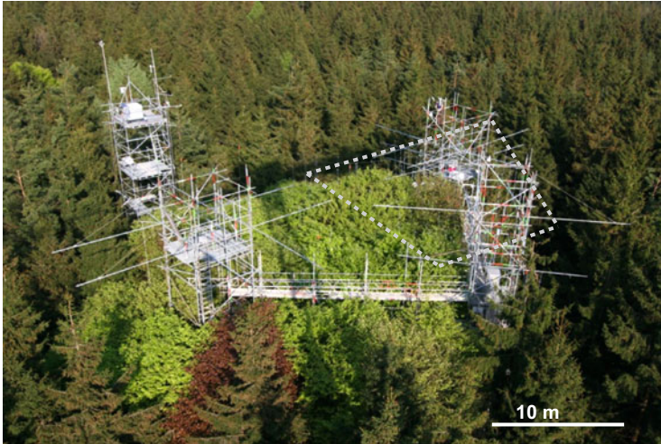
Fig. 11.7 Free-air ozone fumigation experiment at “Kranzberger Forst”, scaffolding consisting of four towers with walkways, May 2006. Ozone was released by a dense gridnet of over 100 teflon tubes hanging from horizontal poles and ropes in the area marked by dotted lines
