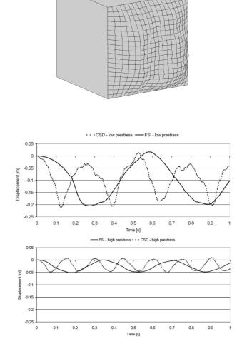
Assuming wind and structural problems to be decoupled leads to very poor calculation of structural dynamics.
