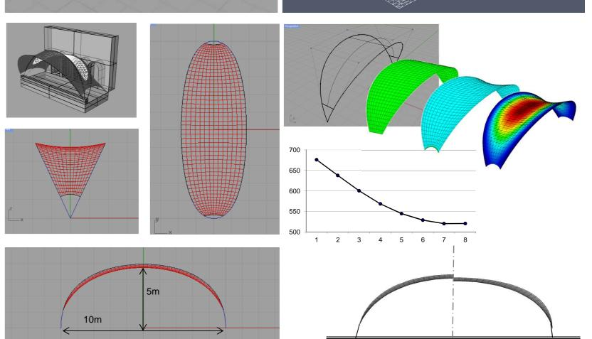
Design chain of a membrane roof. The shape is parameterized by NURBS and form-finding. Optimization is done by a fully coupled sensitivity analysis
