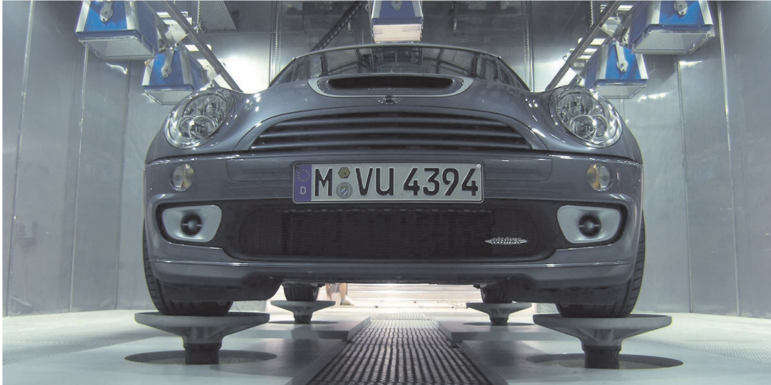
Figure 2.2.: CREST road simulator with hydropulsers, climatic chamber and floodlight system for the imitation of sunlight [53].
