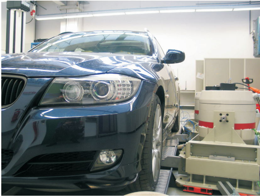
Figure 2.4.: Vibration test rig with electrodynamic actuators [53].
