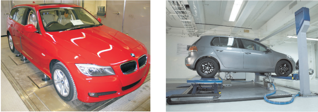
Figure 2.7.: Road simulation with electromagnetic reluctance actuators. Left: test rig with integrated climatic chamber (actuators not visible) [53]. Right: test rig with lifting platform.
