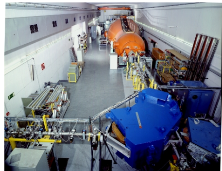
Figure 10.6: Photograph of the Tandem Accelerator tank (orange) and the first deflecting magnet (blue).
