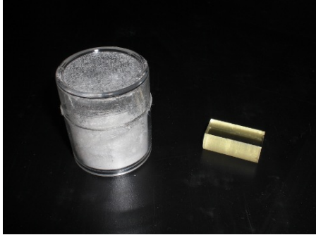
Figure 7.12: Samples of PPO (left, refilled) and acrylic (right) for the NAA.
