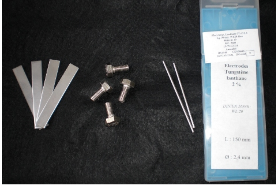
Figure 7.9: Photograph of different material samples from the InnerVeto. From left to right: steel rails, steel bolts (both for holding the VM2000-foil), and the welding electrodes (including its blue plastic wrapping).
