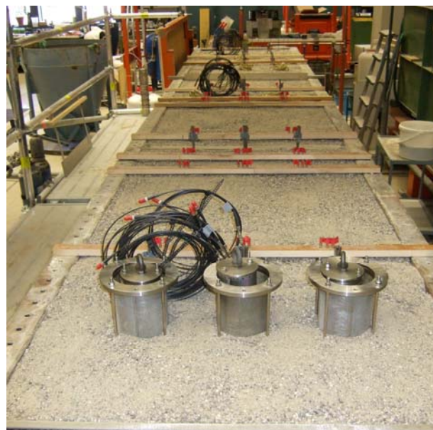
Figure 1.3. View over the mesoscale indoor model aquifer.
