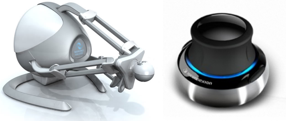
Figure 4.25 Supported force-feedback device with three degrees of freedom and three feedback channels and 6-dof input device.
