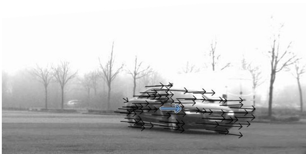
Figure 4.8 Feature based optical flow result: motion field for a moving object and a mean transformation generator projected back into the image.
