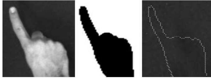
Figure 4.16 Steps to find the contour used for gesture type classification: color-conversion, segmentation, and contour extraction.
