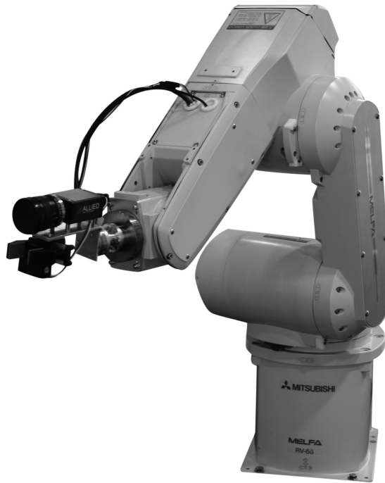
Figure 4.24 An active perception setup implies an actuated sensor device. In the figure, the sensor (a camera) is mounted to the end-effector of a Mitsubishi RV-6S robot.
