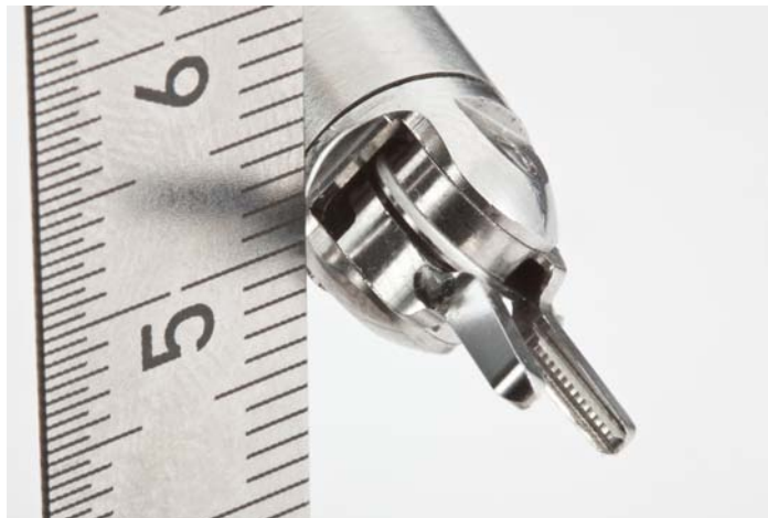
Figure 5.21: Closeup view of the tool tip with short jaws which are used as needle holder. Centimeter scale to the left.
