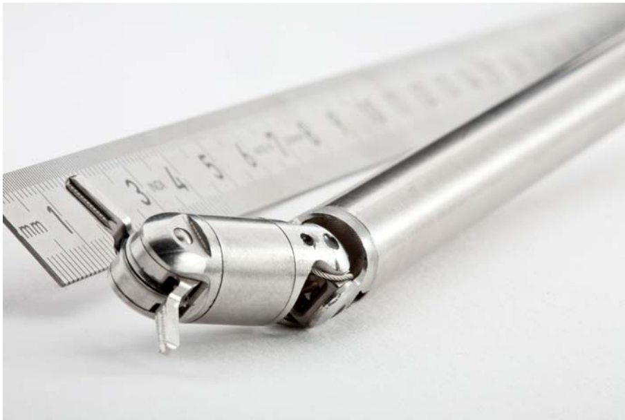
Figure 5.1: Closeup view of the minimally invasive tool tip in the form of a short needle holder with centimeter scale in the background. Diameter of the tool is 10 mm.
