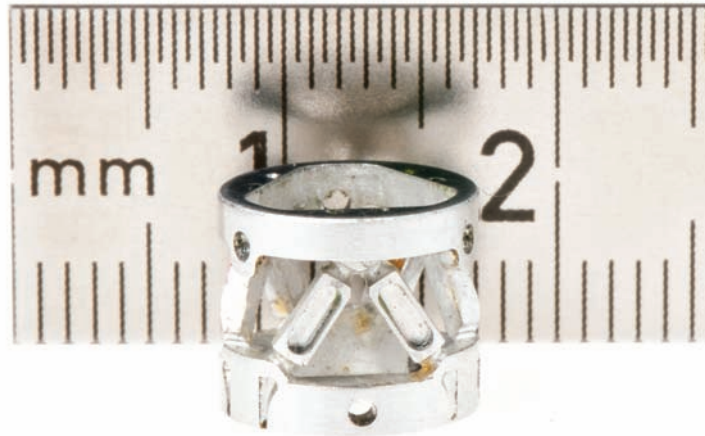
Figure 5.9: Image of first generation monolithic sensor geometry fabricated by milling from Al-CuMg1.5 (F55) aluminum with a diameter of 9.4 mm.
