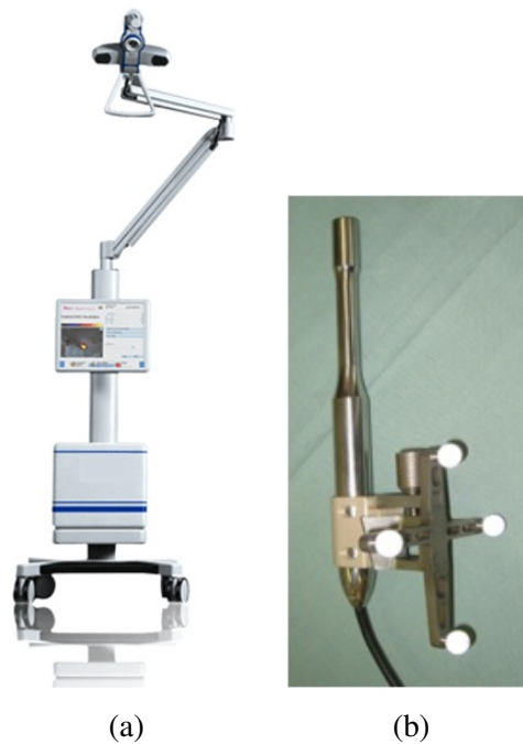
Figure 6.1.: (a) The intra-operative SPECT imaging device, (b) the tracked gamma probe of the imaging device.
