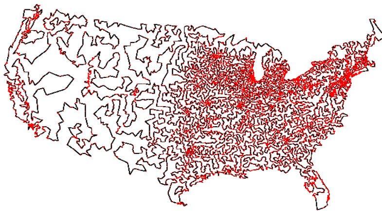
Figure 2.6: Optimal route connecting 13,509 U.S. cities with populations of more than 500 people (GATECH 2005)
