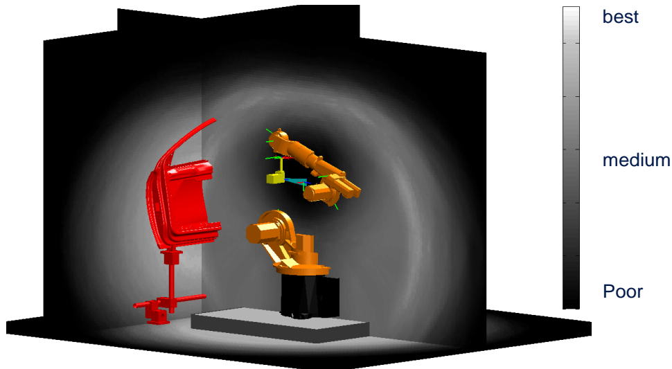
Figure 5.6: Scannability map of an FIS. The map is sliced by two vertical planes for better visualization.
