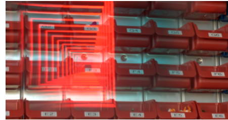
Figure 9: The Tunnel visualization (photographed through the Nomad HMD). The blue shadow originates from the optical combiner of the Nomad.
