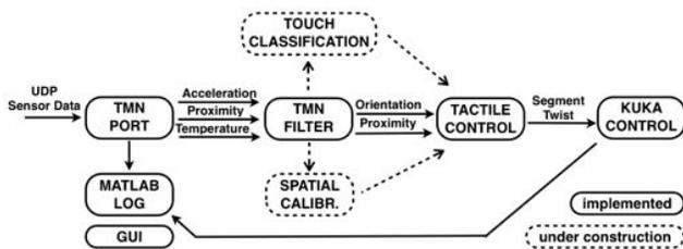
Fig. 6. Schematic overview of the Tactile Computing Cluster
