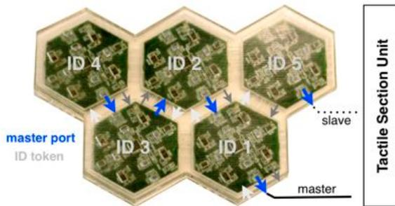
Fig. 5. Example Network Calibration for a Skin Patch
