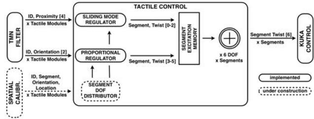
Fig. 7. Schematic overview of the Tactile Controller
