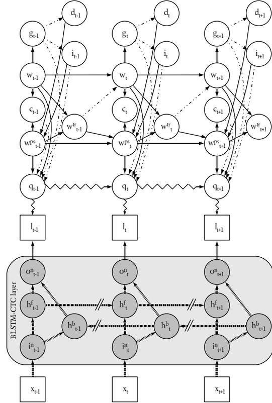
Fig. 2. Hybrid CTC-DBN architecture for keyword spotting
