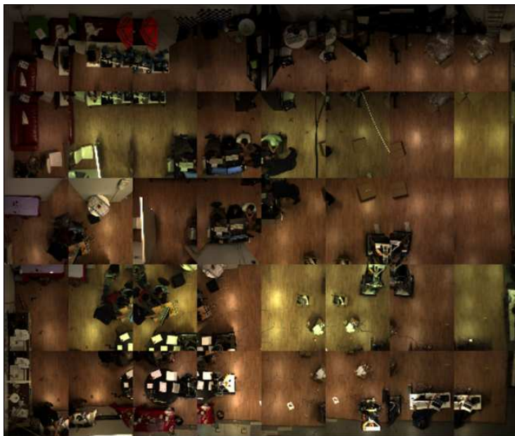
Figure 9: Tiled joint view of the 40 cameras observing the apartment mockup. Different illumination conditions are caused by object shadows, while variant chromatic appearances are caused by using different camera models. Specular reflections result from light sources above the ceiling-mounted cameras.
