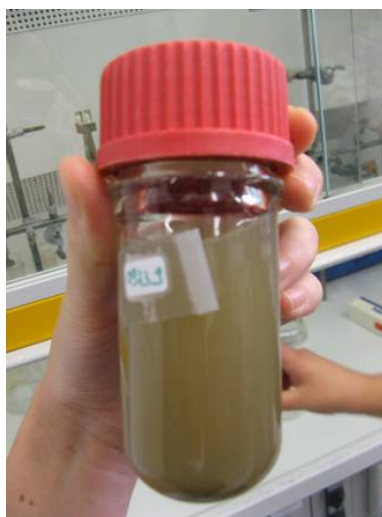
Figure 4. Batch with soil sample used for the phenanthrene sorption experiments.
