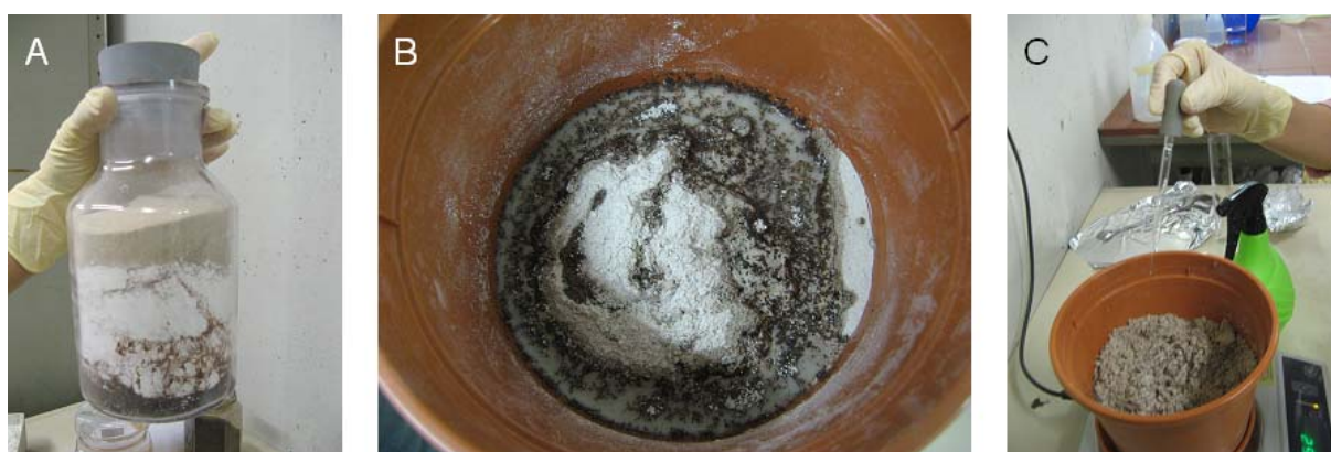
Figure 1. Mixing of the model materials (A, B) and initial wetting of the artificial soil batches.
