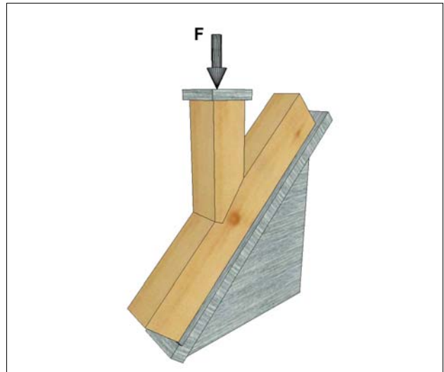
Figure 16: Specimen and Configuration of Experiment for Step Joints (Failure in Compression at an Angle \alpha to the grain)
