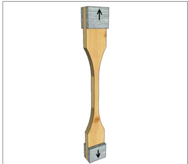
Figure 1: Specimen and Configuration of Experiment for Failure in Tension parallel to the Grain
