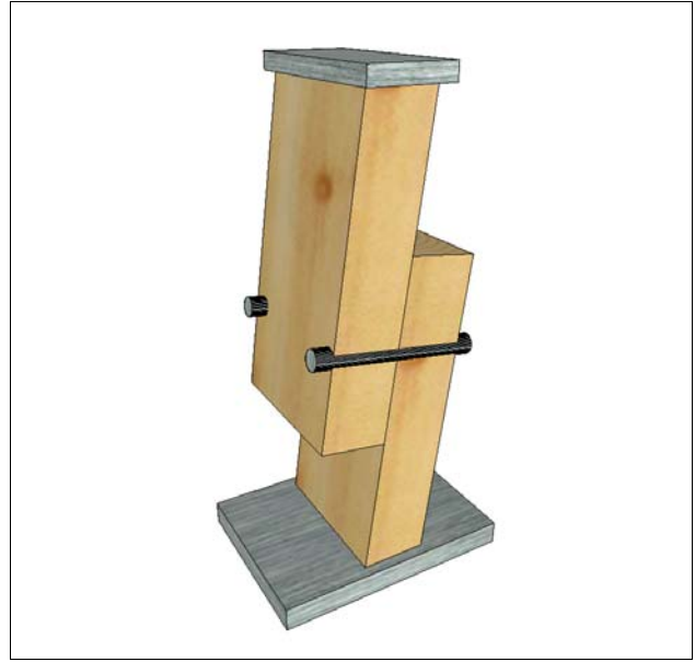
Figure 20: Configuration of Experiment for Embedment Strength failure in a Single-Shear Connection
