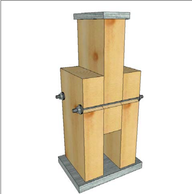
Figure 22: Configuration of Experiment for Yielding Failure of Bolts in a Double-Shear Connection including the Rope Effect
