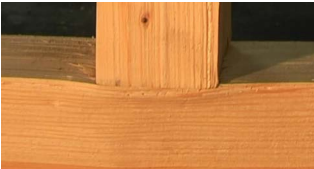
Figure 15: Detail of Specimen failing in Compression perpendicular to the Grain
