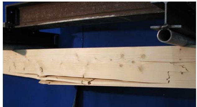
Figure 6: Detail of Specimen failing in Bending (Tension failure parallel to Grain)
