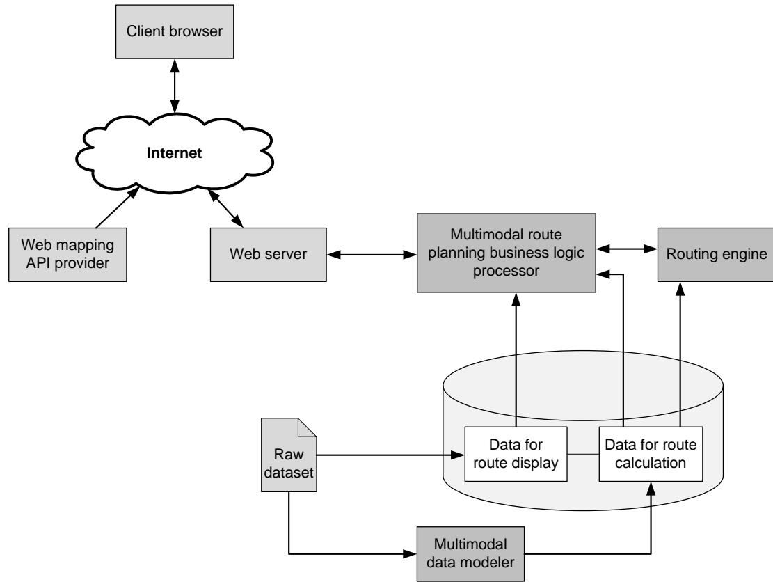
Figure 5.4     Architecture of the prototype system.
