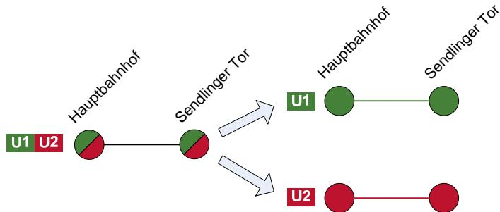
Figure 3.9 Separation of underground lines U1 and U2 between Hauptbahnhof and Sendlinger Tor stations.
