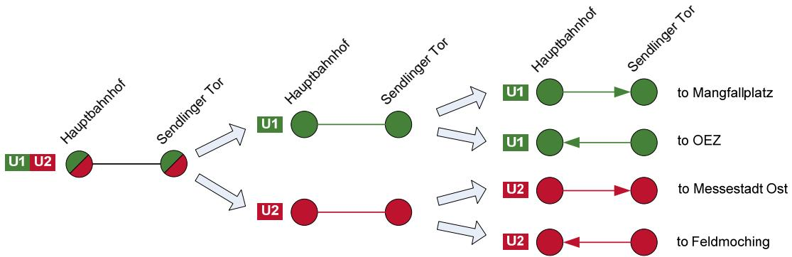
Figure 3.11 Separation of underground lines U1 and U2 between Hauptbahnhof and Sendlinger Tor according to their different heading directions.
