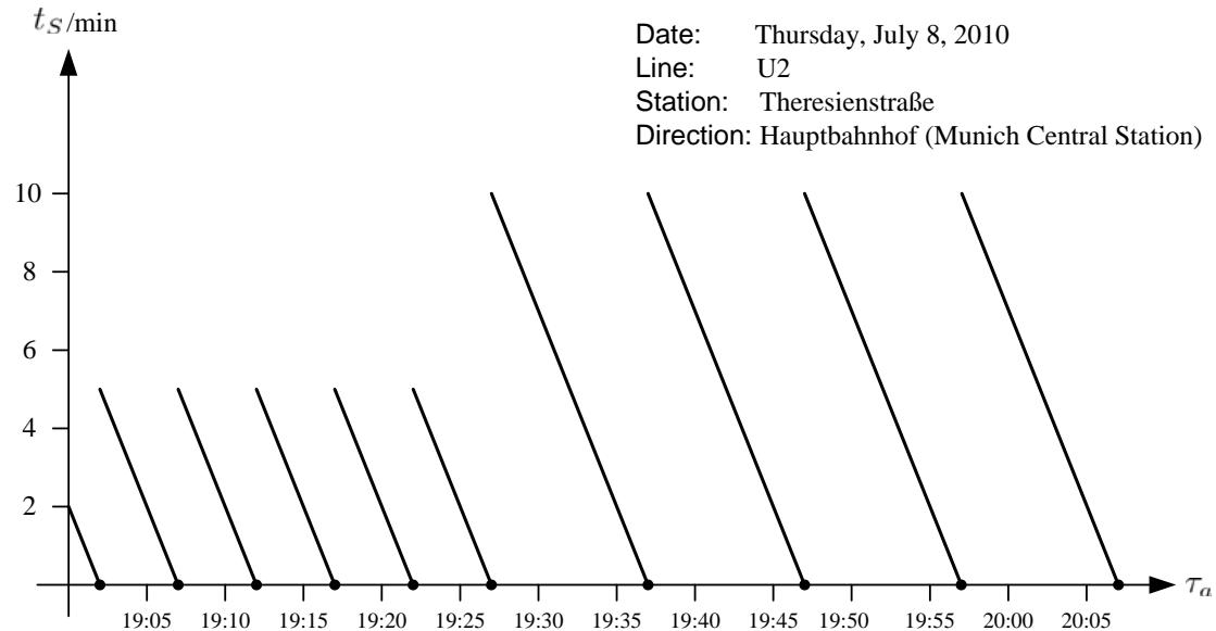
Figure 3.15 Piecewise linear function of waiting time at Theresienstraße station of underground line 2 on Thursday, July 08, 2010 according to the timetable in Figure 3.14. The underground train comes every five minutes from 19:02 to 19:27, and every 10 minutes from 19:37 to 20:07.
