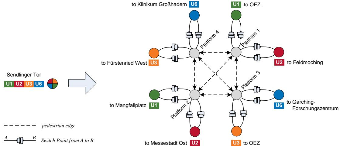
Figure 3.21 Switch Points at underground station Sendlinger Tor.
