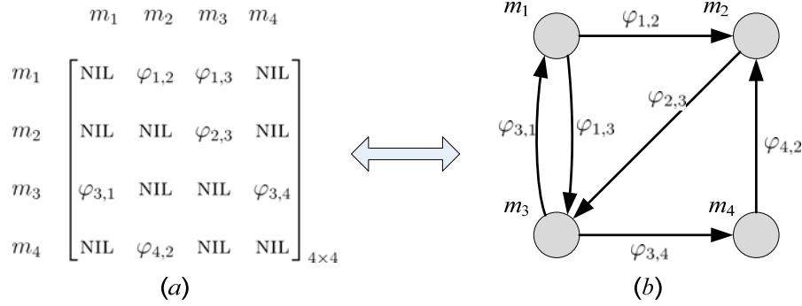
Figure 4.1 An example of Switch Condition Matrix (SCM) and the expressed graph.
