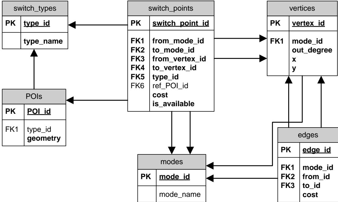
Figure 5.2 Entity-Relationship diagram of multimodal routing database.
