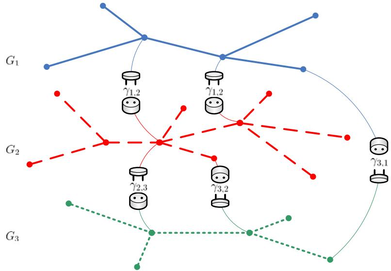
Figure 3.23 Example of one-way and double-way pluggable graphs.
