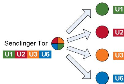
Figure 3.8 Separation of Sendlinger Tor station into four vertices belonging to U1, U2, U3 and U6.
