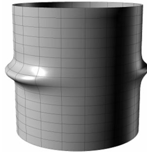
Figure 9.7: The optimized geometry from Figure 9.6(b) as design geometry in a CAD environment.
