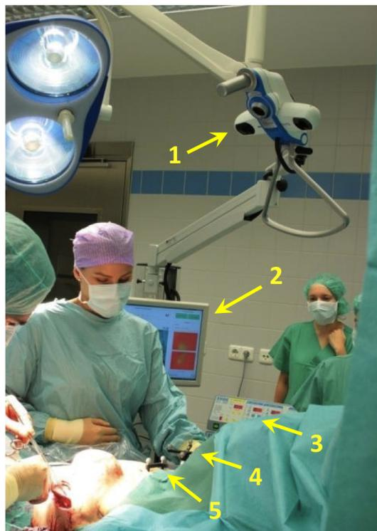
Figure 5.16: Freehand SPECT system in intra-operative setting consisting of (1) infrared tracking system, (2) touch screen monitor for display and interaction, (3) a hand-held gamma probe with mounted tracking target and (4) a patient tracking target to determine the position of the patient in a common coordinate system.
