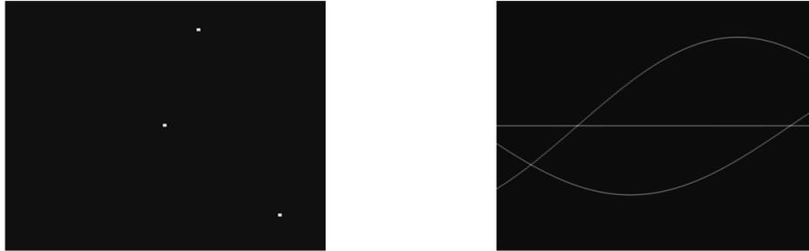
Figure 2.2: *Left:* image with three points, *right:* sinogram of those three points created using a parallel scanning geometry.
