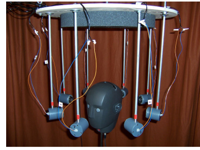
Figure 3: Circular loudspeaker array with 8 speakers; the distance between the speaker membrane and the ear canal entrance measures 15 centimetres.
