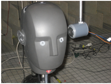
Figure 2: HRTF measurements in the near-field, here at a distance of 6cm between the loudspeaker membrane and the entrance to the ear canal.
