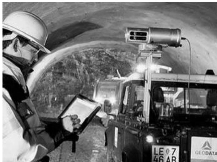
Figure 3: Driving-attendant laser scanning with the Orthos Laser Tunnel Scanner [6]
