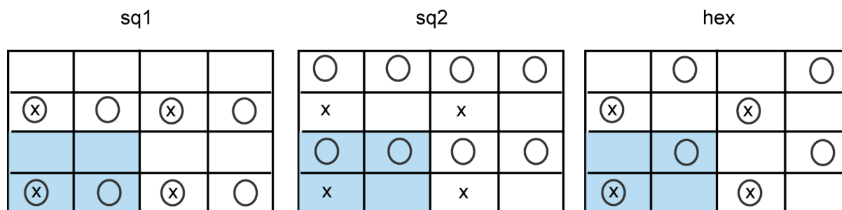
Figure 8.3. Schematic representation of positions of two silanol defects in the (2 \times 2) unit cell (shaded) of a kaolinite slab. Adsorption complexes of uranyl at an AlOO site are indicated by a crosses, circles represent the positions of the defect groups: sq1 – square lattice of defect positions below the surface (uranyl is adsorbed directly above one of them); sq2 – square lattice of defect positions below the surface. Uranyl is adsorbed between two defects; hex – defects of a hexagonal lattice (uranyl adsorption above the defects).
