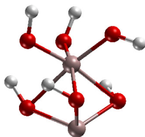
Figure 8.4. Cluster model \text{Al}_2(\text{OH})_6 used to estimate deprotonation energies of aluminol groups.
