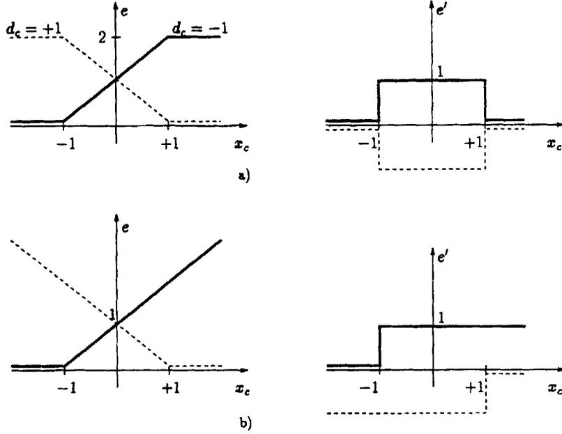
Figure 3. (a) Conventional and (b) state-based error measure and its derivative
