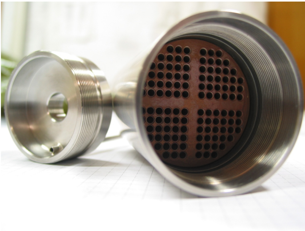
Figure 4.5: Heat exchanger inside the ^3\text{He} evaporation stage. Right: copper plate with hole array inside the stainless steel housing of the evaporation stage. Left: bottom flange of the exchange volume, which will be connected to the converter volume via a copper tube in “U”-shape.
