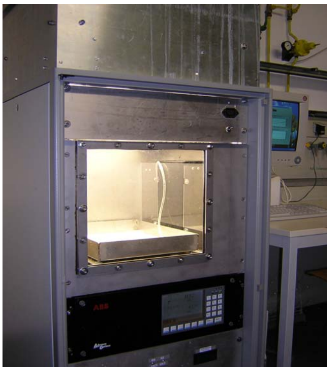
Figure 32. The chamber for incubation of plants with ^{13}\text{CO}_2 .
