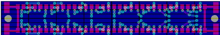
**Figure 8.5:** Detail from the four-layer readout PCB, showing a group of 64 signal pads (dark blue), which are connected by displaced vias (light blue) to the soldering pads (violet) of one high-density SMD connector. All layers are shown overlaid. Only 64 out of the 68 connector pins are used for signal readout, the remaining four for grounding purposes.
