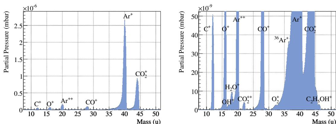
**Figure 8.9:** Left: mass spectrum of the Ar/ $\text{CO}_2$  gas mixture used for the TPC operation, obtained by a quadrupole spectrometer. Right: same spectrum, but zoomed on the  $y$  axis to enlarge small components. For both plots, the black points indicate the step size during the spectrometer scan.
