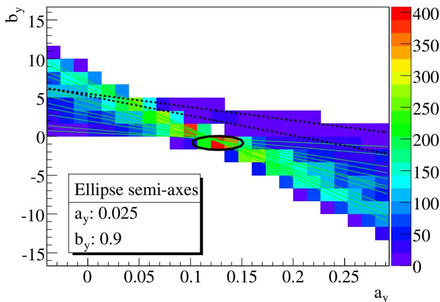
**Figure 8.27:** Pattern recognition in the TPC test chamber using the method of Hough transform (see text). An ellipse around the center of the bin with the maximum accumulated line length (indicated by the color scale) selects “hits-on-track” (green lines intersecting the ellipse). Outliers (black dashed) are rejected for the track fitting; same event as in figure 8.25.
