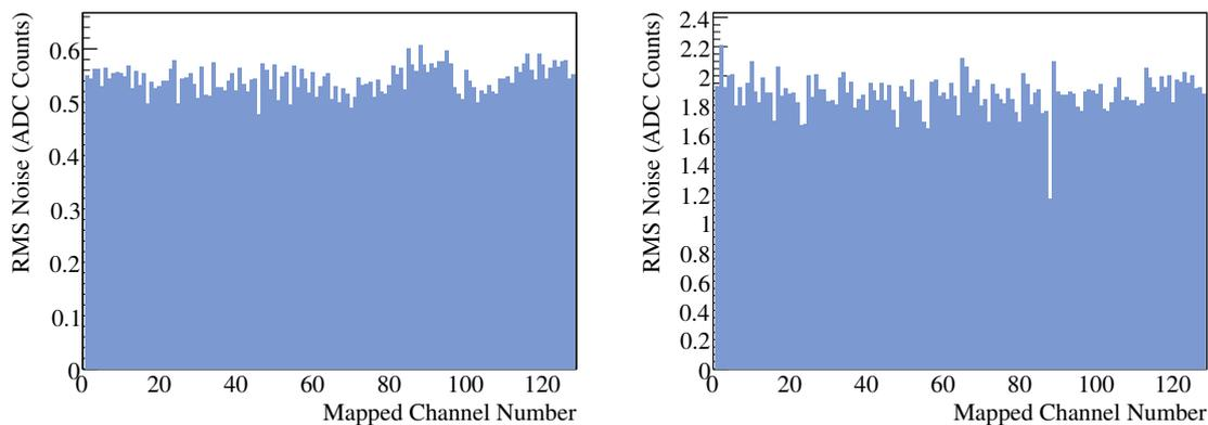
**Figure 8.21:** Noise performance of the TPC readout electronics, RMS for each channel shown. The 128 channels are mapped “left to right” if looking from the front to the SPI. Left: only ALTRO card connected, average noise 0.54 ADC counts. Right: everything including TPC connected and powered, average noise 1.88 ADC counts.
