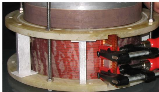
**Figure 8.10:** Schematic detail of the field cage, showing the connection of the inner and outer strips via the resistor chain.
