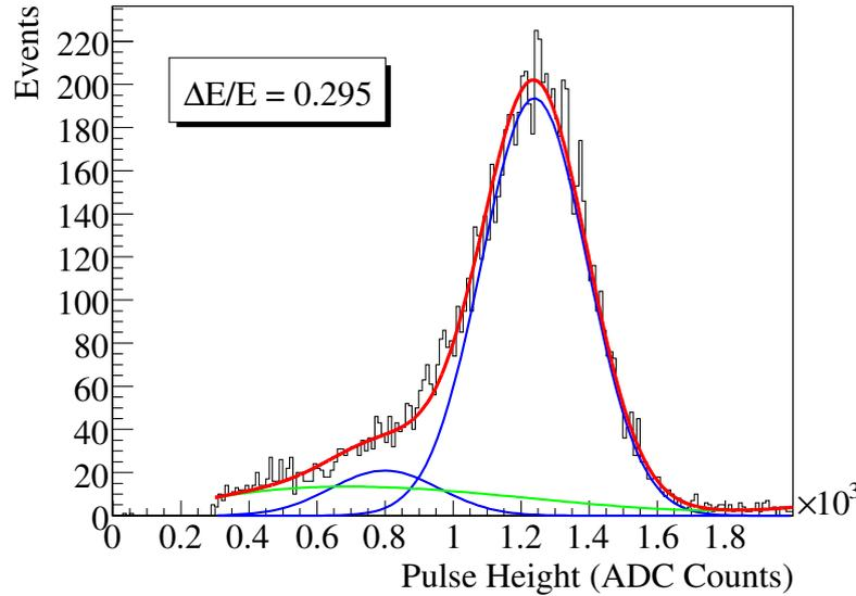
**Figure 8.17:** TPC pulse height spectrum recorded with copper X-rays. The red curve displays the result of a fit with two single Gaussians (blue) and some background polynomial (green). Resolution obtained from “photo peak” (FWHM).
