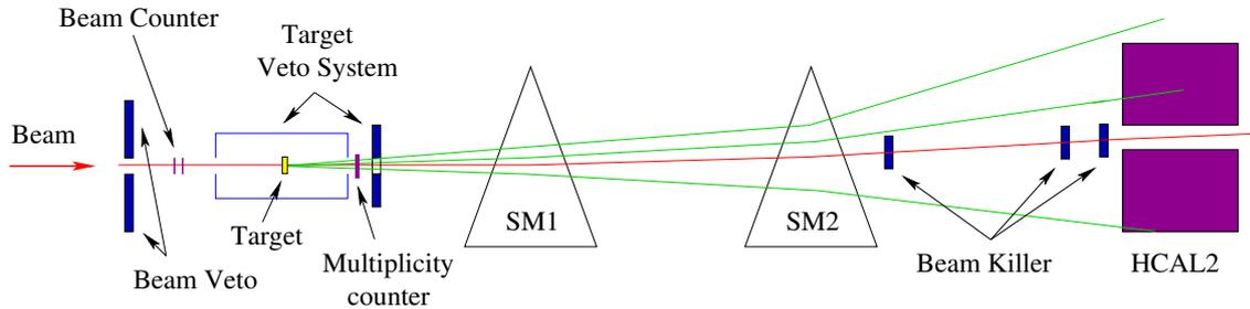
**Figure 3.3:** Sketch of the 2004 diffractive trigger scheme (see text); veto components are drawn in blue, others in magenta. Shown are a  $3\pi$  event (green lines) fulfilling all trigger requirements and a single pion event (red line) corresponding to a non-interacting beam particle; the latter case is vetoed by the beam killers.
