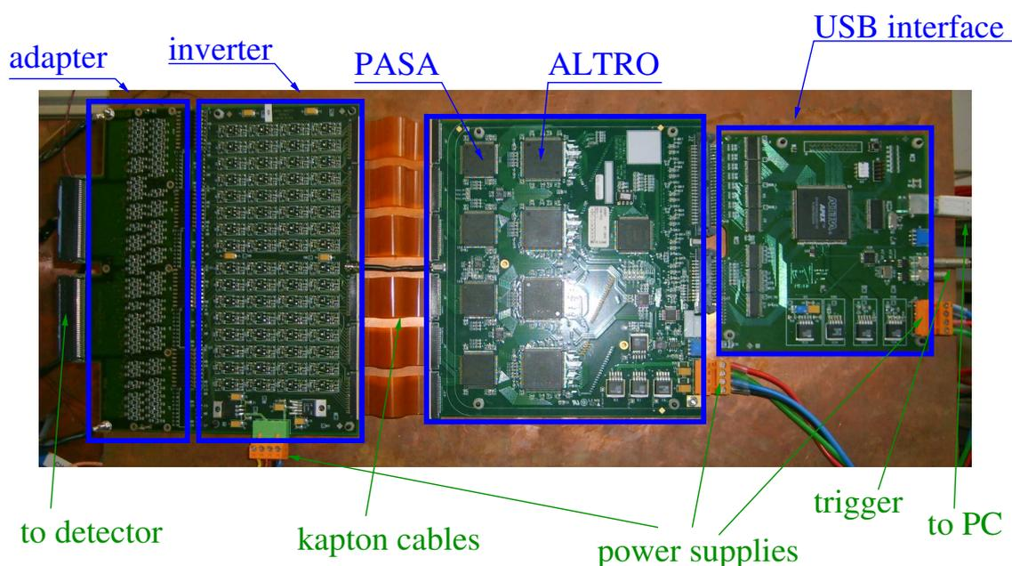
**Figure 8.20:** Overview photograph of the test chamber readout electronics chain. The basic processing elements are labeled in blue, while the green captions point out interfaces and connectors. All cards are mounted to a copper support plate.
