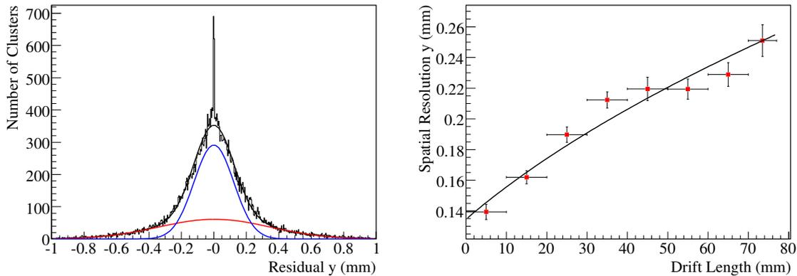
**Figure 8.30:** Left: Residual distribution of  $y$  coordinate for standard settings (see text). A double-Gaussian fit to the data is presented in black; the blue and red curve show the two single Gaussians. Right:  $y$ -resolution dependence on the drift distance  $z$ ; horizontal error bars indicate the width of the eight defined  $z$ -regions. The black curve represents a fit to the data according to equation (8.2).
