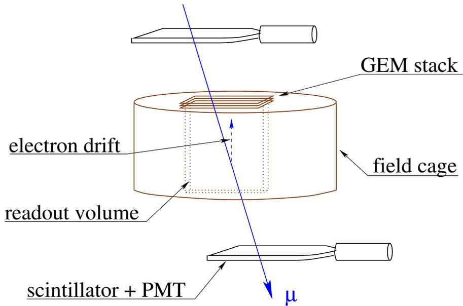
**Figure 8.22:** Position of trigger detectors with respect to the test chamber; TPC mounted horizontally (drift direction vertical), thus muons cross the readout plane and the GEM stack rather perpendicularly. The sensitive volume of  $99.2 \times 8 \times 77 \text{ mm}^3$ , given by the area of the read out pads and the drift length, is indicated.
