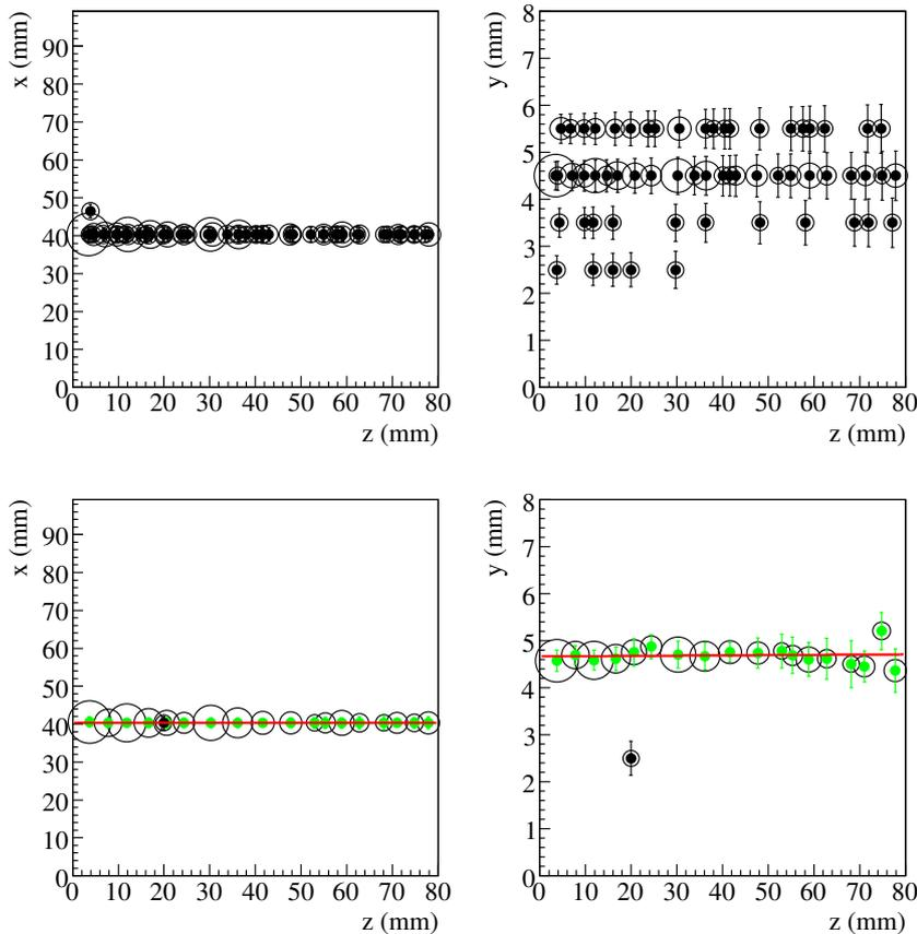
**Figure 8.26:** Cosmic muon event in the TPC test chamber; perpendicular angle of incidence w. r. t. the pad plane. See caption of figure 8.25.
