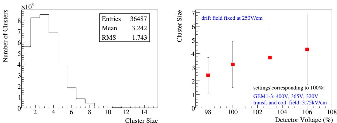
**Figure 8.29:** Left: Distribution of sizes of 3-dim. clusters for standard settings (“100%”). Right: Mean cluster size for different GEM stack settings, RMS of each corresponding distribution drawn as error bar.
