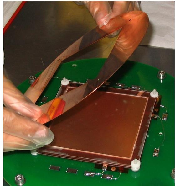
**Figure 8.6:** Detail of the readout plane showing part of the signal pads, three HV feedthroughs and one sink hole for a GEM stack pillar.
