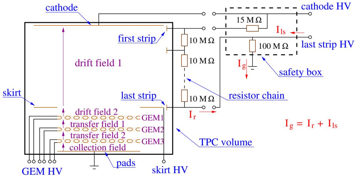
**Figure 8.8:** Overview of the test chamber high voltage system including the definition of the adjustable electrical fields (magenta color); HV connectors are marked as circles. Currents through resistor chain  $I_r$  and from last strip supply  $I_{ls}$  sum up to ground current  $I_g$ ; e. g. for  $U_c = 6$  kV and  $U_{ls} = 3$  kV:  $I_c = 8$   $\mu$ A and  $I_{ls} = 22$   $\mu$ A, cf. figure 8.12.
