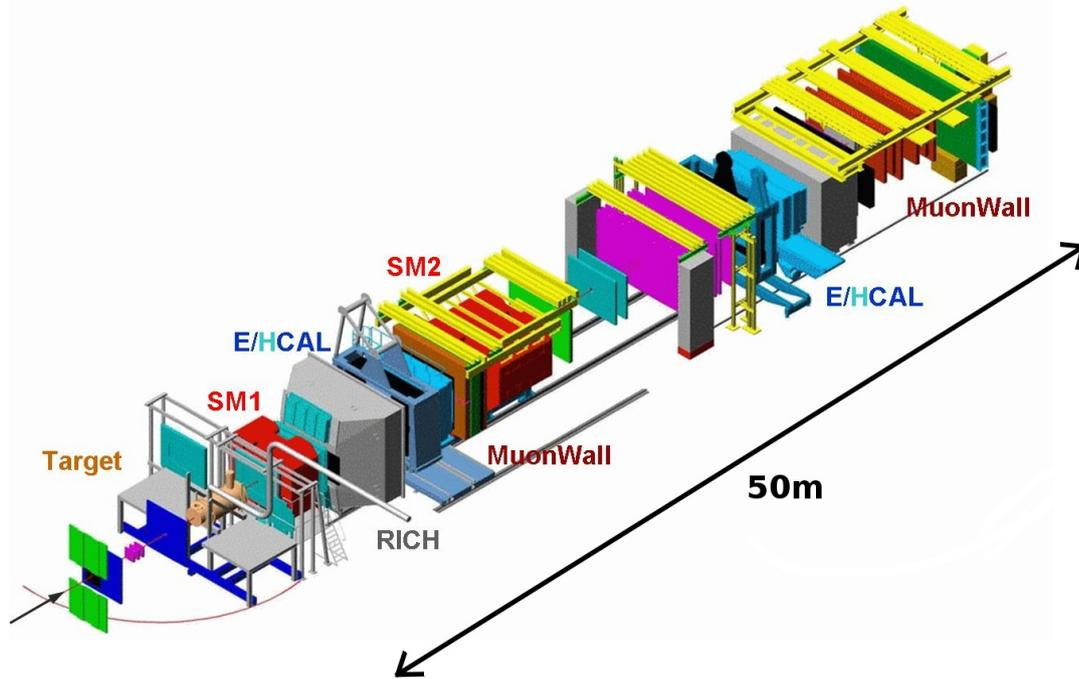
**Figure 3.1:** Artists view of the COMPASS experiment at CERN; setup corresponding to data taking with the polarized target (light brown color) shown. The beam is coming from the left. For further details see text and [14].
