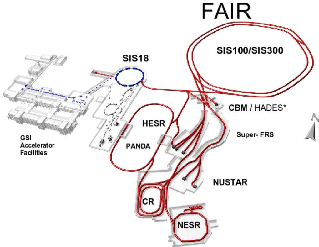
**Figure 6.1:** Schematic layout of the present GSI facilities (left, blue color) and the planned FAIR complex (right, red color). The PANDA experiment will be located at the antiproton storage ring HESR.
