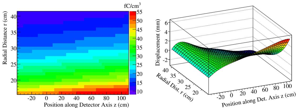
**Figure 7.2:** Simulated ion space charge density inside the PANDA TPC (left) and resulting radial displacements of drifting electrons depending on their  $rz$  start position (right) [189]. The readout end-cap is located in the plane  $z = -40$  cm.
