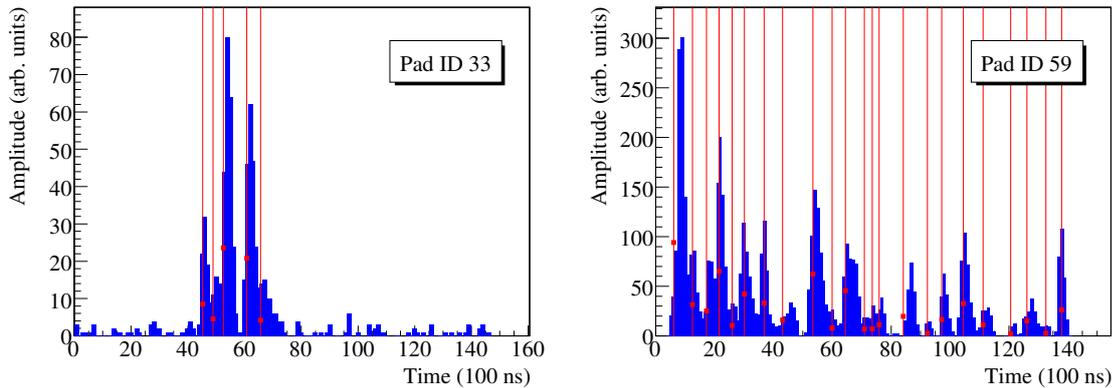
**Figure 8.24:** Time structure of the charge (blue, ADC units) as induced on a readout pad for one complete electron drift time. The situation of an oblique (left) and a perpendicular (right) muon track is compared. A pulse shape analysis performed for both pads yields a time (indicated by the red vertical lines) and an integrated amplitude (scaled down by a factor of 10, indicated by the red markers) for every pulse.
