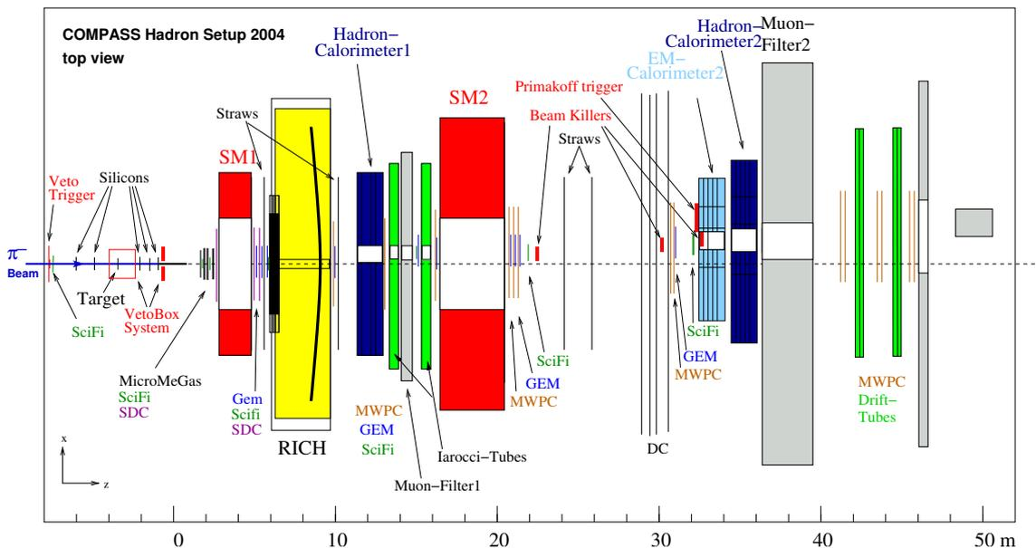
**Figure 3.2:** Schematic view of the COMPASS pilot hadron run setup in 2004 (without beam line); spectrometer magnets indicated in red color. For details on the different components (including their abbreviations) see text and [14].
