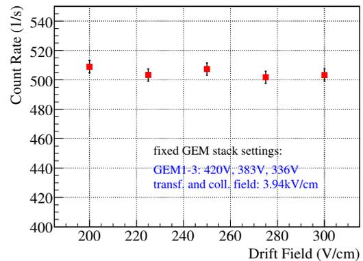
**Figure 8.16:** X-ray count rate vs. drift field; GEM stack settings fixed to “105%” (inside efficiency plateau). Errors are statistical.
