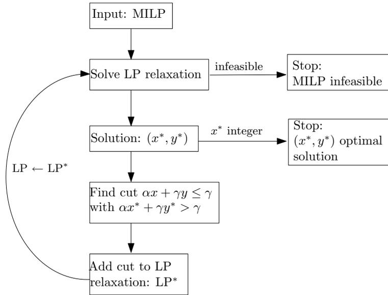
Figure 1.1: The basic principle of a cutting plane algorithm according to [Pad05]
