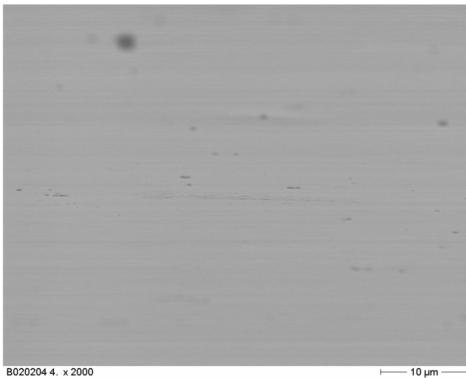
Fig. 53: SEM picture of the surface of the sample PET 23 SiO 2 020204 (2000x)
