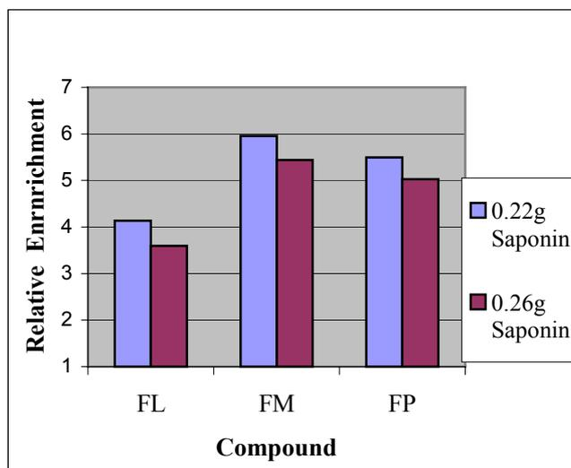
**Figure 4.2** Enrichment of Fradiol Esters by Foam Fractionation, in Dependence of Saponin Concentration in the Initial Solution
