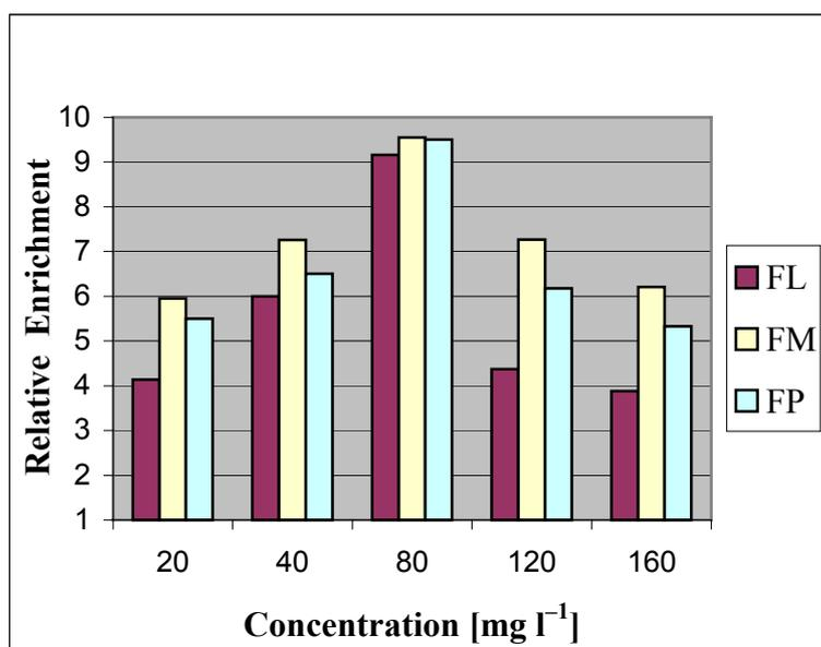
**Figure 4.3** Enrichment of Faradiol Esters by Foam Fractionation, in Dependence of their Concentration in the Initial Solution
