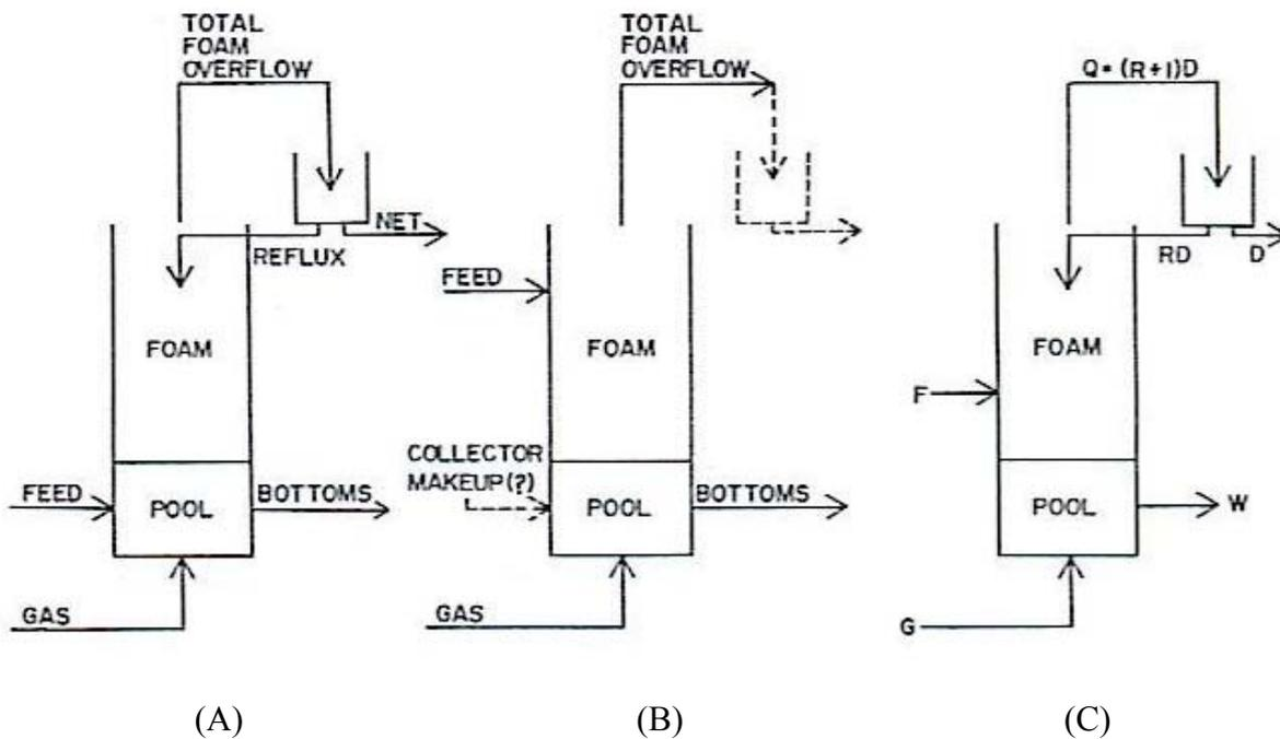
**Figure 2.9** Foam Fractionation in a Continuous Process. (A) Enrichment Mode. (B) Stripping Mode. (C) Combined Mode (Lemlich, 1972a)
