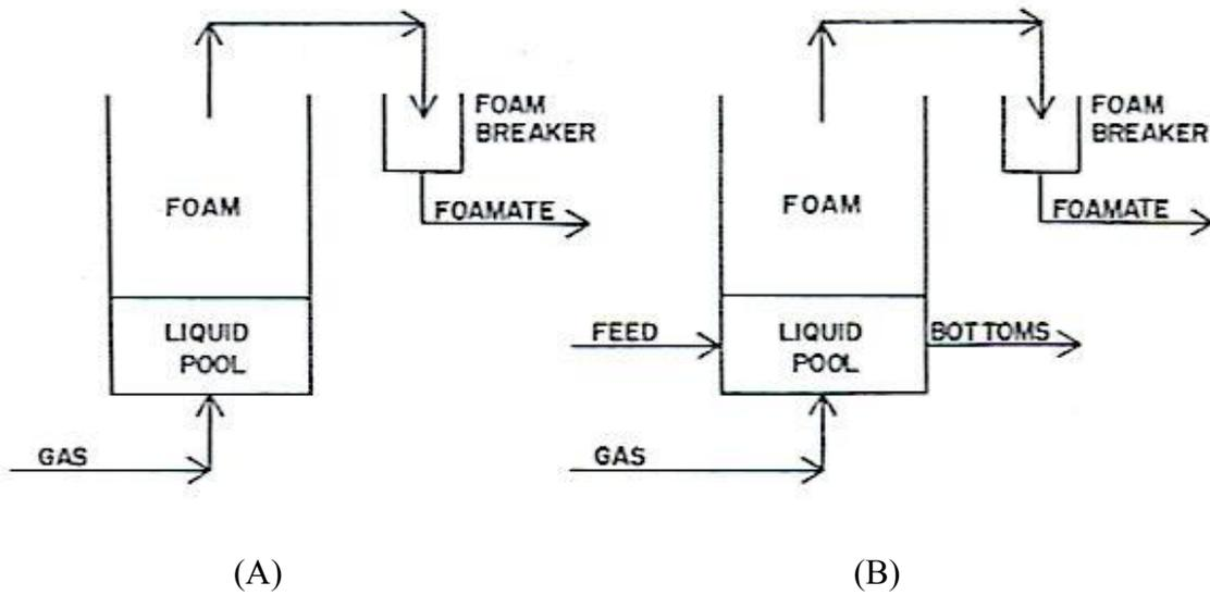
**Figure 2.8** Foam Fractionation in the Simple Mode: (A) Batch Process. (B) Continuous Process (Lemlich, 1972a)
