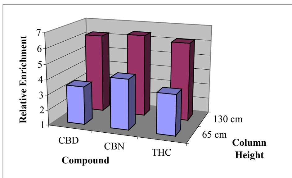
**Figure 4.24** Enrichment of Cannabinoids by Foam Fractionation, in Dependence of Column Height
