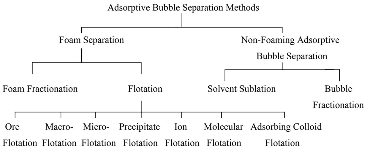
**Figure 2.1** Schematic Representation of Adsorptive Bubble Separation Methods (Karger *et al.*, 1967)
