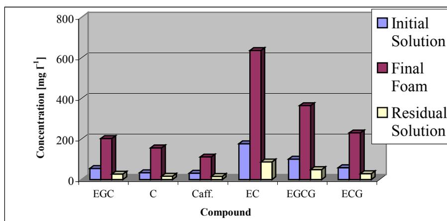
**Figure 4.11** Concentration of Catechins and Caffeine in the Initial Solution, Overall Foam and Residual Solution, for the Foam Fractionation Process
