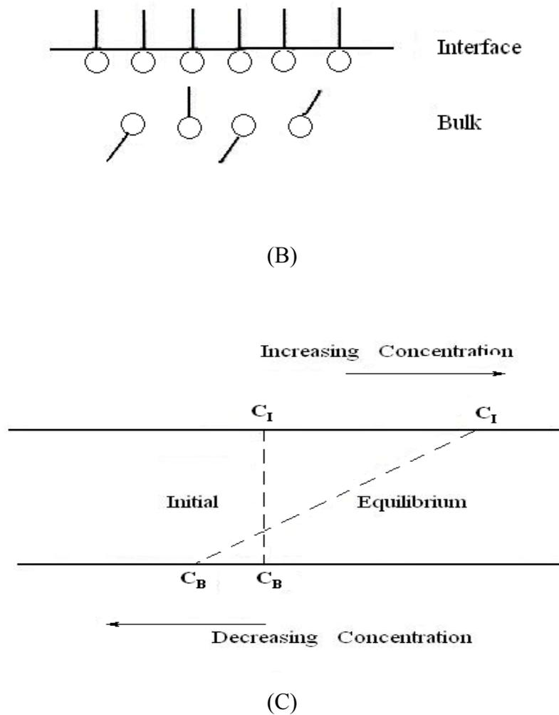
**Figure 2.3** Representation of Interface and Bulk Phase Concentration Resulting from Adsorption, During the Foam Fractionation Process (Charm, 1972 ; de Vries, 1972) (A) Initiation of the Process. (B) Equilibrium. (C) Whole Process.  $C_I$  – Concentration at the Interface.  $C_B$  – Concentration at the Bulk. (○—) Surfactant. (○) – Surfactant Hydrophilic Part (—) Surfactant Lipophilic Part
