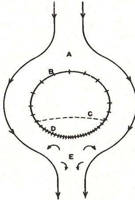
**Figure 2.4** Adsorption at the Surface of a Bubble Rising Inside a Liquid Pool. A: Upstream Region; B: Bubble; C: Separation Ring; D: Crowding of Adsorbed Material; E: Wake (Lemlich, 1972c)
