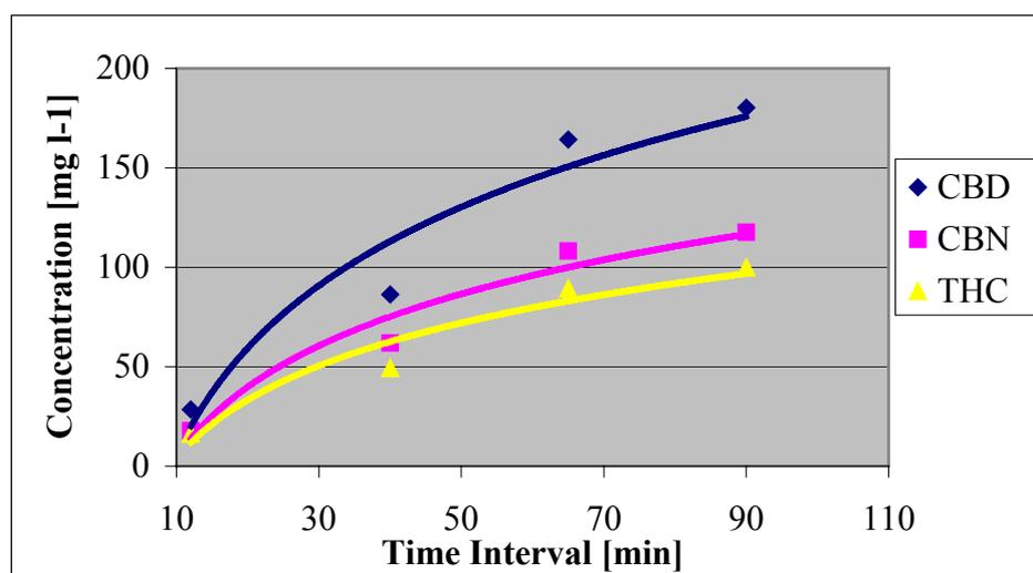
**Figure 4.25** Increase of Cannabinoids Concentration from Initial Solution, to Foam Collected Along the Consecutive Foam Fractionation Process
