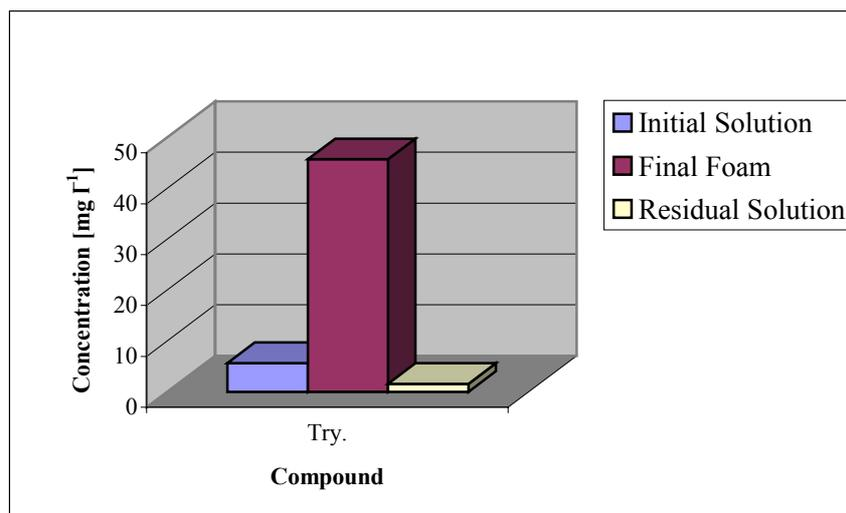
**Figure 4.19** Concentration of Tryptanthrin in Initial Solution, Overall Foam and Residual Solution, for the Foam Fractionation Process
