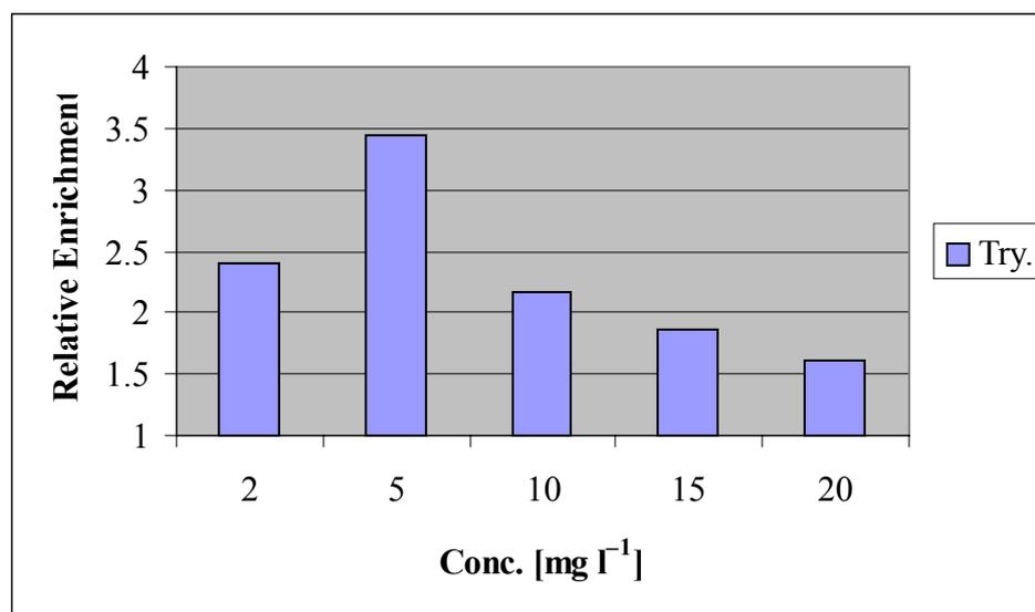
**Figure 4.15** Enrichment of Tryptanthrin by Foam Fractionation, in Dependence of its Concentration in the Initial Solution
