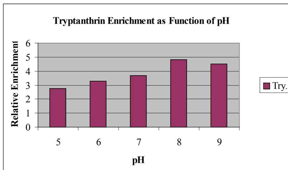
**Figure 4.16** Enrichment of Tryptanthrin by Foam Fractionation , in Dependence of Initial Solution pH
