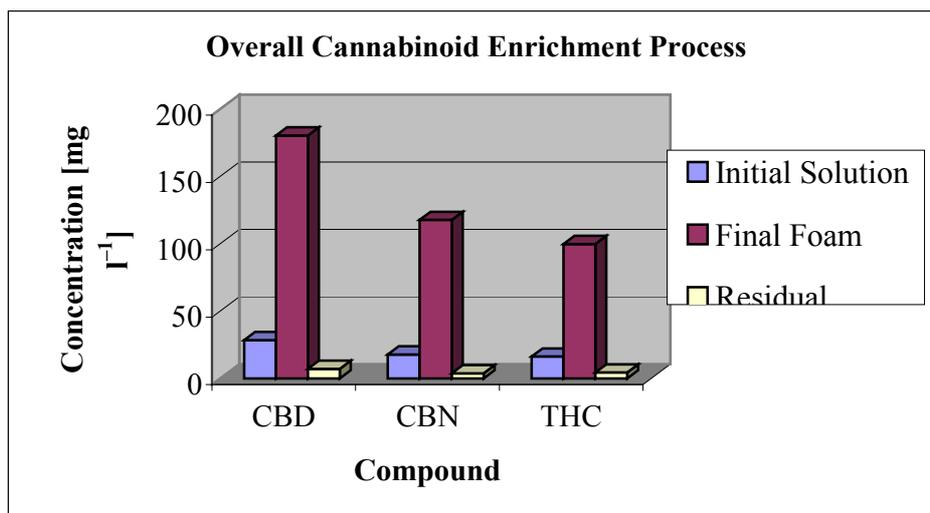
**Figure 4.26** Concentration of Cannabinoids in the Initial Solution, Overall Foam and Residual Solution, for the Foam Fractionation Process
