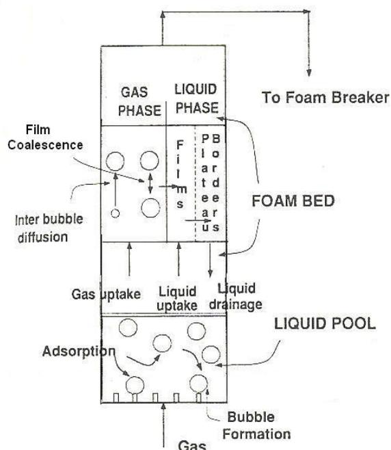
**Figure 2.7** Schematic Diagram of the Phenomena Occurring in a Fractionation Column (Uraizee and Narsimhan, 1996)
