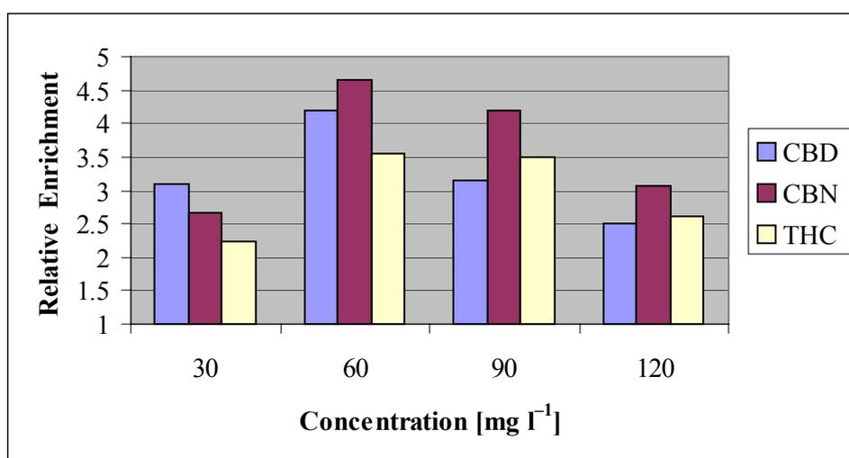
**Figure 4.22** Enrichment of Cannabinoids by Foam Fractionation, in Dependence of their Concentration in Initial Solution
