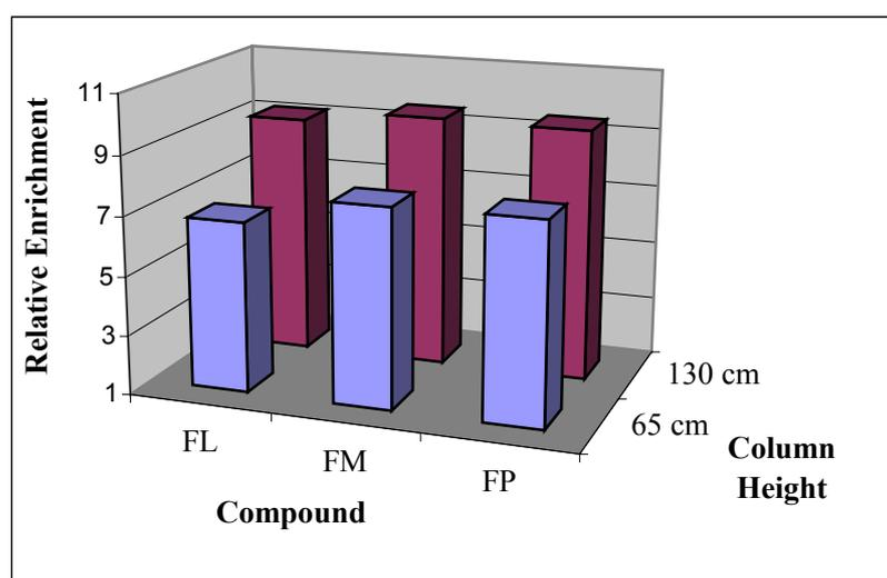
**Figure 4.4** Enrichment of Faradiol Esters by Foam Fractionation, in Dependence of Column Height
