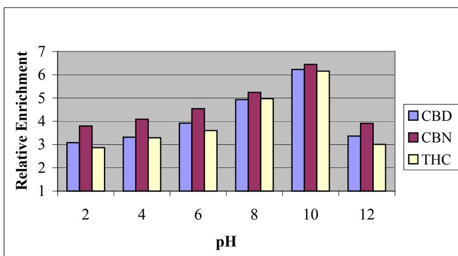
**Figure 4.23** Enrichment of Cannabinoids by Foam Fractionation, in Dependence of Initial Solution pH
