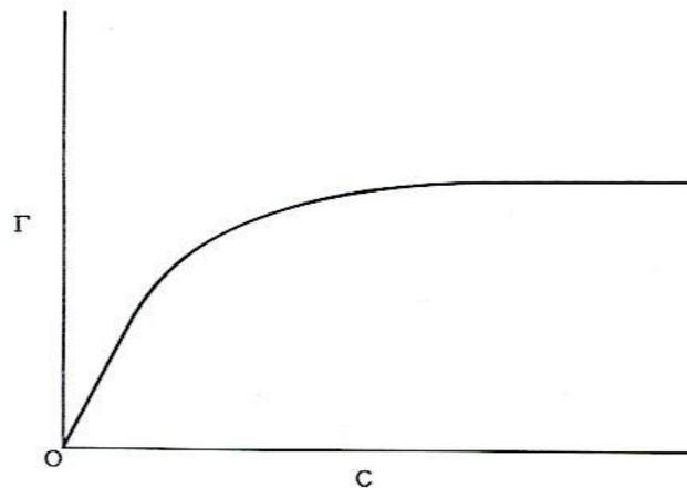
**Figure 2.2** Curve Showing the Effect of Solute Concentration in Solution on the Solute Concentration at the Surface for the Adsorption Process (Lemlich, 1972a)
