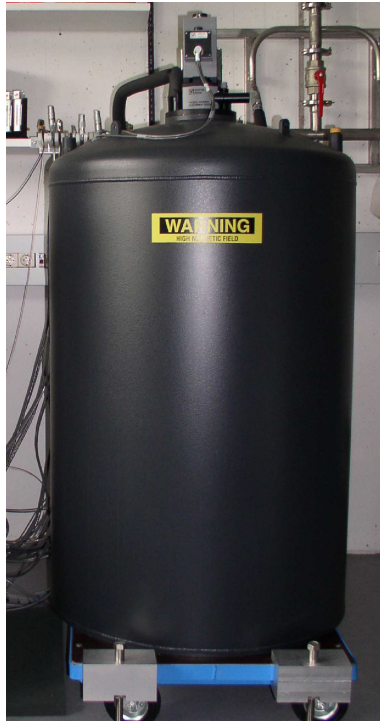
Figure 3.1: Left figure: The Physical Property Measurement System (PPMS, Quantum Design, Inc.) allows for a temperature range of 1.8 K to 400 K with an external vertical field from zero Tesla to \pm 9 T. Figure above: straw sample holder, in which a solid or powder sample is placed and that would be loaded into the sample chamber.
