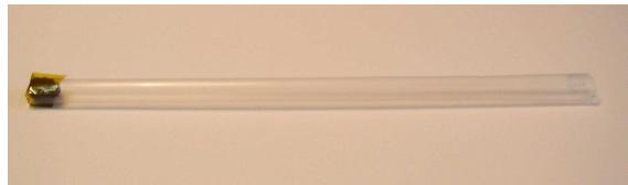
Figure 3.1: Left figure: The Physical Property Measurement System (PPMS, Quantum Design, Inc.) allows for a temperature range of 1.8 K to 400 K with an external vertical field from zero Tesla to \pm 9 T. Figure above: straw sample holder, in which a solid or powder sample is placed and that would be loaded into the sample chamber.
