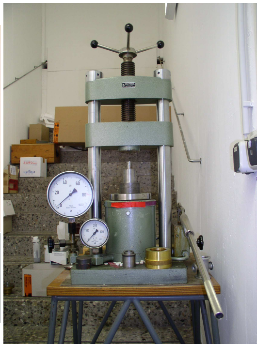
Figure 4.1: Technical equipment that was used during the sample synthesis process at the Walter Meissner Institute. Left figure: Mortar with basin and crucible for grinding the components into fine powder and heating up the pellets in the oven. Right figure: Moulding press for pressing the loose powder into pellets.
