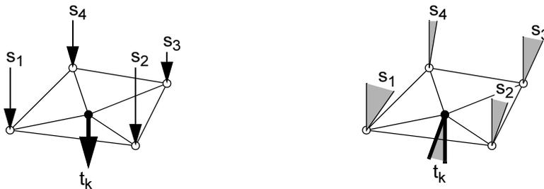
**Figure 6.2** Interpolation of Four Source Points  $s_i$  to a Target Point  $t_k$  (Non-Conservative)
