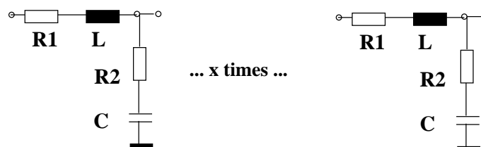
Fig. 5.21: Equivalent circuit model (or finite network model) of a tube. Each R_1 L C R_2 - element represents a slice of the tube with a certain thickness \Delta x .
