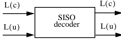
Figure 3.1. Soft-in/soft-out decoder with soft-output information about code bits.
