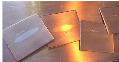
Figure 3.2: Miniplates manufactured at CERCA for heavy ion bombardment
