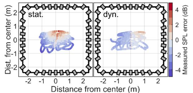
**Figure 2:** Dynamically measured broadband SPL errors inside the loudspeaker array with HOA playback. Each dot represents a microphone position, the color indicating SPL error. The left panel shows the static EQ and the right panel shows the dynamic EQ.
