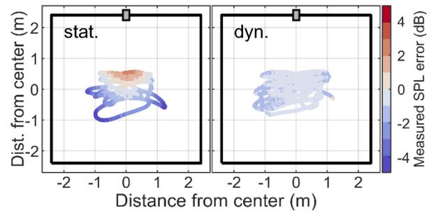
**Figure 1:** Dynamically measured broadband SPL errors inside the loudspeaker array with single loudspeaker playback. Each dot represents a microphone position, the color indicating SPL error. The left panel shows the static EQ and the right panel shows the dynamic EQ.
