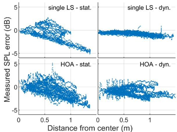
**Figure 3:** SPL errors for different EQ and playback methods as a function of distance from the center of the loudspeaker array.
