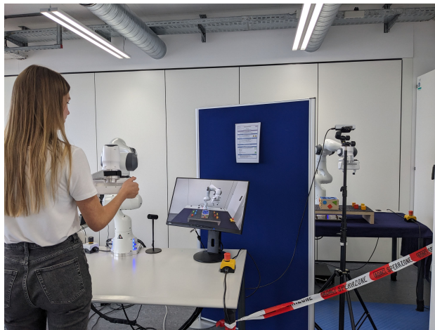
Figure 6 An image of a participant operating the teleoperated system with a monoscopic 2D screen
