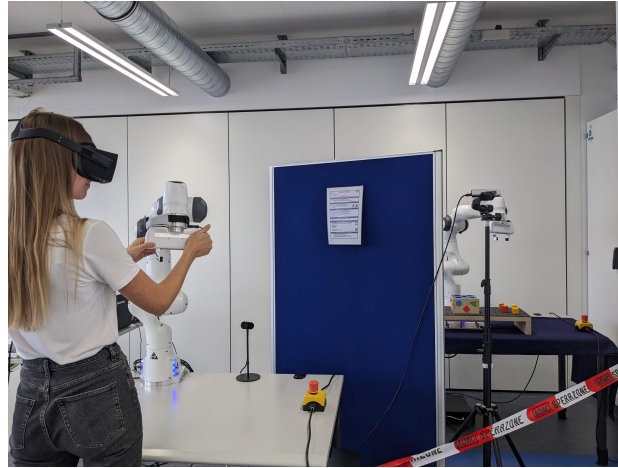
Figure 7 An image of a participant operating the teleoperated system with either a monoscopic or stereoscopic display on the HMD
