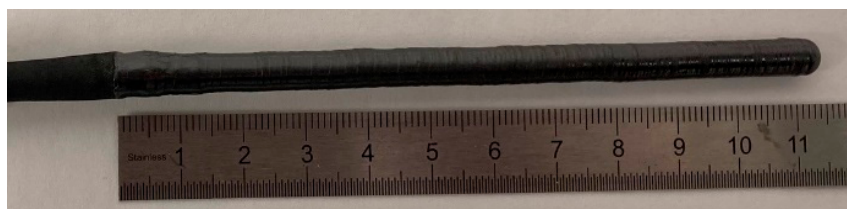
Figure 2. As-grown \text{Nd}_{1.3}\text{Sr}_{0.7}\text{NiO}_{4+\delta} single crystal as obtained by floating zone method by using a mirror furnace (NEC-SC2).
