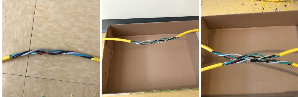
Figure 6. Photos of applied degradations (Left) at Spot B after execution of Stage 3, (Middle) at Spot A after execution of Stage 5, (Right) after execution of Stage 7.
