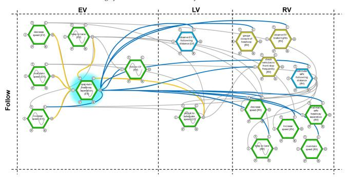
**Figure 13.** The critical path of the function < maintain headway separation (EV) > for the human driver.
