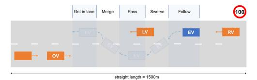
**Figure 2.** Schematic illustration of the overtaking scenario comprising different road users/agents and divided into five temporal and spatial stages. EV = ego vehicle, LV = lead vehicle, RV = rear vehicle, OV = oncoming vehicle.
