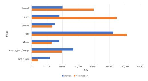
Figure 9. Comparison of the GSV for the overall system and per stage between human and automation.
