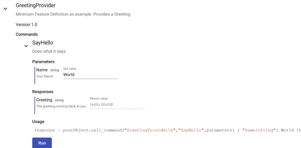
Fig. 4. The bottom layer of the service tree allows direct execution of command and property calls. If no parameter is supplied for command calls, the default parameter will be used. In case of device services, accidental execution may have serious unwanted consequences; thus, execution must be confirmed.
