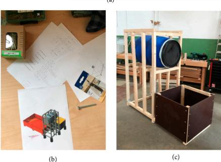
**Figure 10.** Documentation of the development of technical components for the BGA project. (a) Considerations for septic tank design and filter loading. These students' sketches do not show the final design, but an intermediate step in the planning. (b) Based on CAD drawings and 3D models, the assembly of the components was prepared. (c) The timber framework is pre-fabricated in the workshop.
