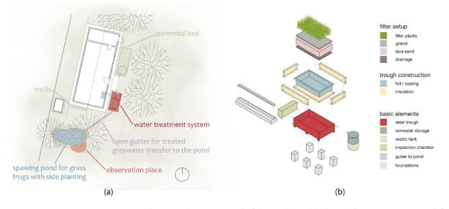
**Figure 9.** Preliminary design proposal of the students. (**a**) The single components were defined and brought into a spatial context. (**b**) The students' axonometry shows the design of the filtration bed. The structure is based on other small greywater treatment plants (examples for comparable structures: [37,41,45]).
