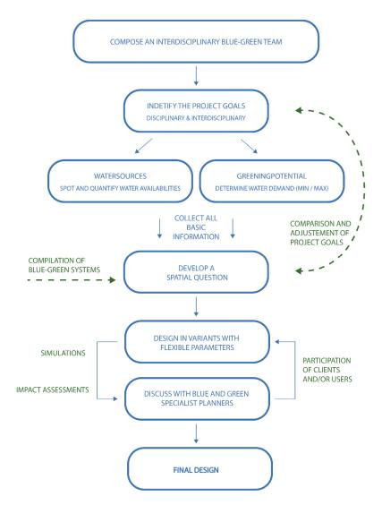
**Figure 16.** The design strategy for blue-green architecture was evaluated through its application in the presented project. In the course of planning and design, weaknesses emerged that should be considered in a revision. The lessons learned and considerations for possible points of intervention are shown in green.
