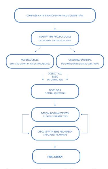
**Figure 2.** Integrated design strategy for blue-green architecture [14]. The integrated planning approach has been developed in a previous design-based research project. The different steps are described in detail in the indicated reference. The design strategy for BGA is applied for the first time in this study. The design process for the BGA project is guided by this approach in order to achieve a balanced weighting of blue and green aspects.
