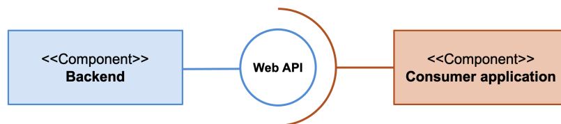
Figure 4.1.: A Web API makes functionality and data accessible to API consumers via the HTTP protocol.
