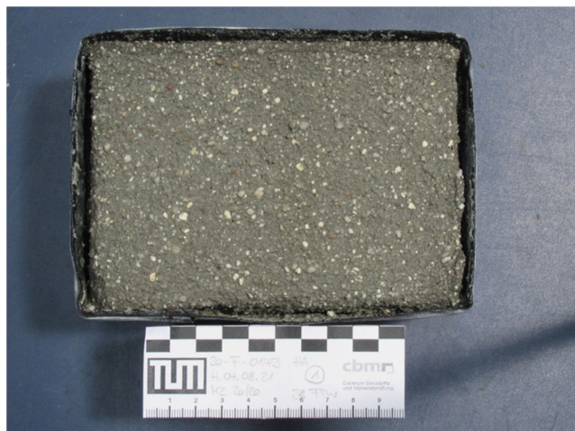
Figure 2. CDF sample showing the detachment of the isolation tape.
