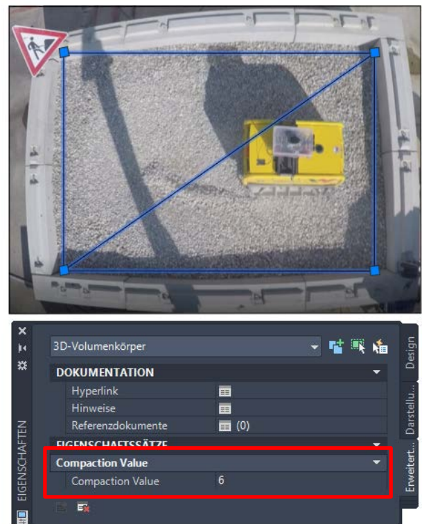
Figure 8: Digital terrain model with compaction factor as input
