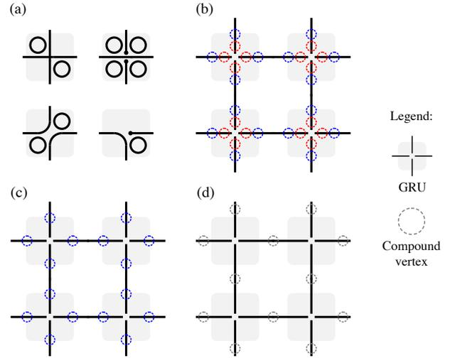
Figure 8. (a) Example GRU configurations. (b) Location of the eight compound vertices on a GRU: four internal vertices (in red) and four port vertices (in blue). (c) Removing internal vertices. (d) Merging port vertices. Final result has up to  $4\times$  lower vertex count for GRU-based designs.
