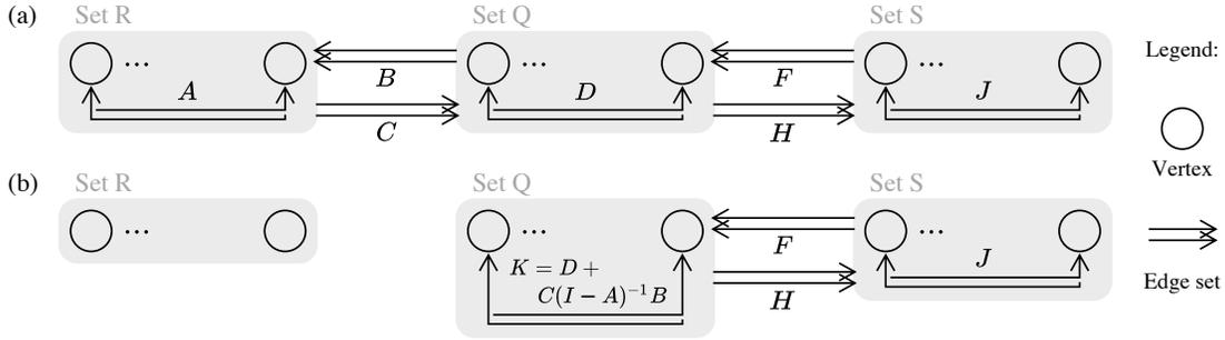
Figure 2. Simplifying a flow graph by removing all edges connected to vertices in the set  $R$ . Each set of edges shown is associated with the corresponding sub-matrix of the transfer matrix  $T$  of the flow graph. (a) Before simplification. (b) After simplification.
