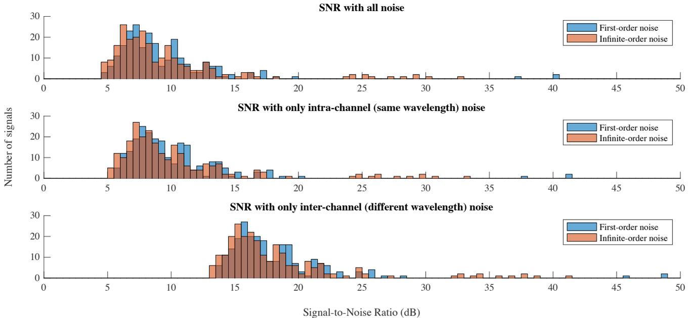
Figure 9. Histogram of SNR results for all 240 signals of a 17 wavelength passive ONoC router.
