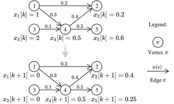
Figure 1. Example of how energy is propagated through the flow graph over one time step, as described by eq. (3).
