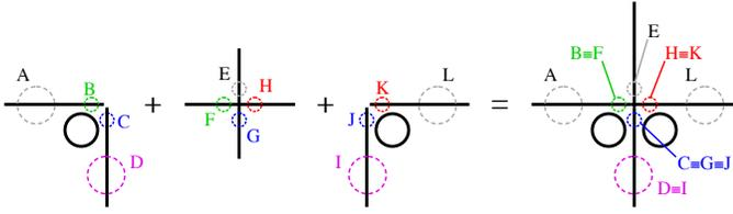
Figure 7. Example of how the compound vertices of isolated elements shown in fig. 6(a) are merged to form a flow graph of an ONoC. In this case, the four compound vertices of two MRRs each and the four compound vertices of a waveguide crossing are combined into a total of seven compound vertices.
